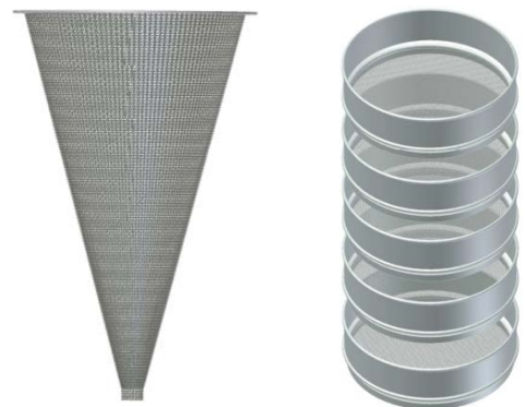
Active sampling insets such as cylindrical nets and cascaded sieves with different mesh sizes
